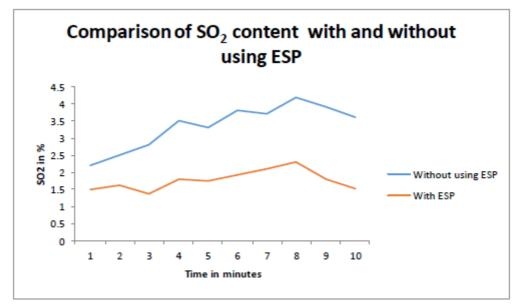
Figure 6. Graphical output of SO<sub>2</sub> content
