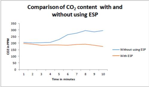
Figure 7. Graphical output CO<sub>2</sub>
