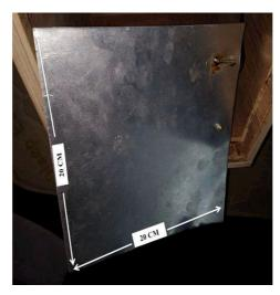
Figure 3. Collection electrodes
