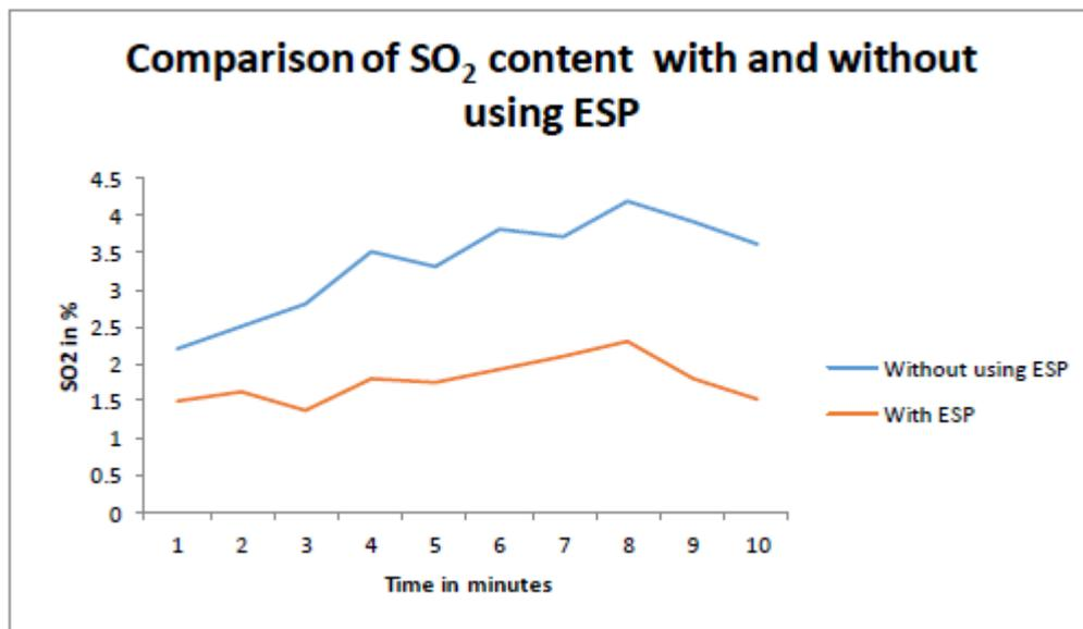
**Figure 6.** Graphical output of SO<sub>2</sub> content
