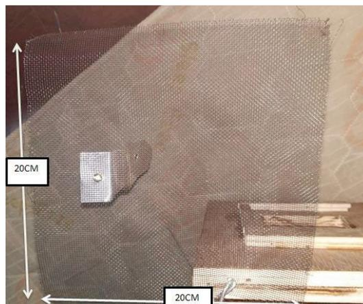
**Figure 2.** Discharge electrodes
