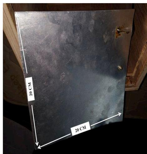
**Figure 3.** Collection electrodes
